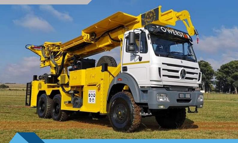
Heavy duty Track or Truck mounted, for Reverse Circulation or Grade. Control Supplied complete with basic set equipments, including on board Air Compressor.
